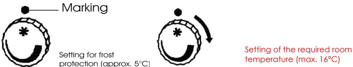
To set the required room temperature: turn the knob in the direction of the arrow to the right as far as it will go (ca. <math>\angle 90^\circ</math>) and wait until the required temperature has been reached. Turn the knob then slowly back again until the control lamp has been extinguished. The position of the knob now corresponds to the required temperature.
